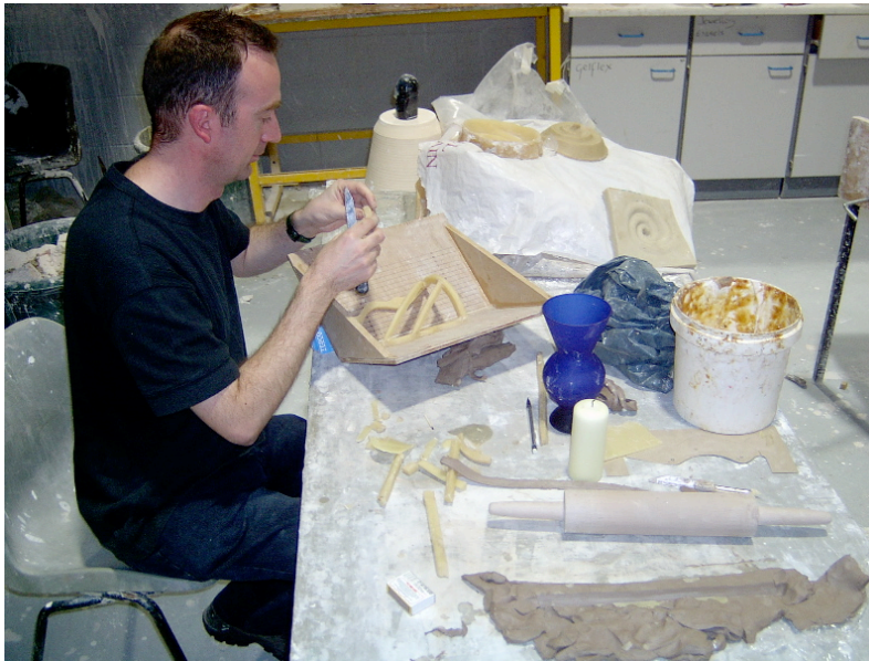
Fig 3. Anthony Pollock preparing a wax model to cast in glass
